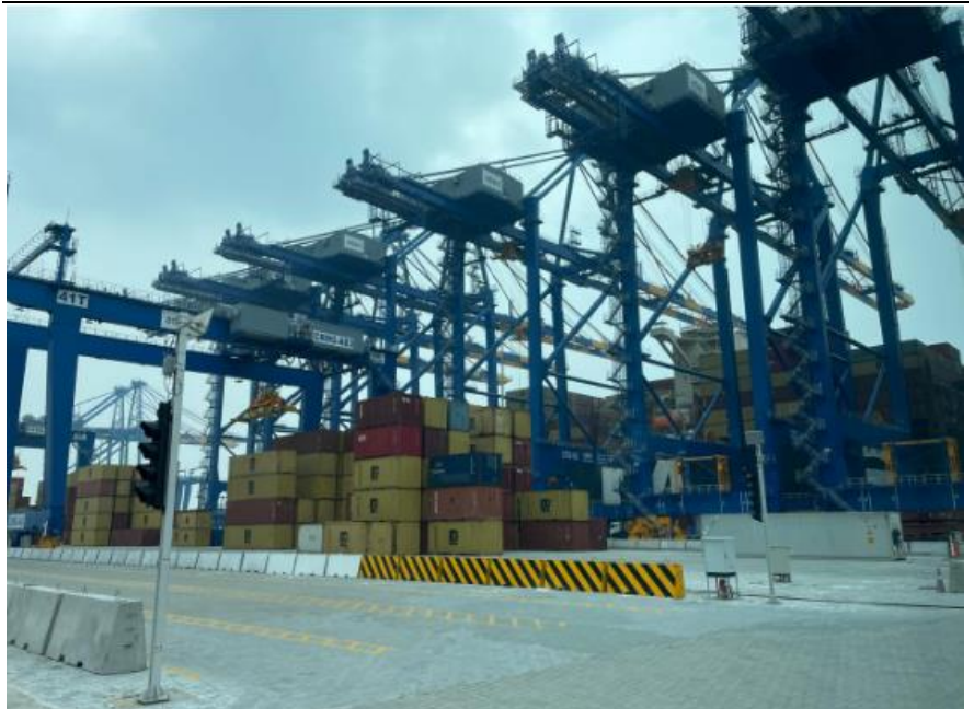
Exhibit 6: Automatic stacking cranes for precision loading and unloading
